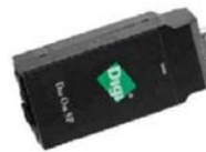
Terminal server to monitor inverters over Ethernet Manufacturer / type Digi One SP
